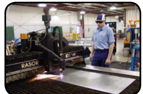
CNC Plasma cutting provides precision parts.
